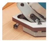
Equipped with front protector to avoid to damage the skirtings or any other element fixed on the wall.
