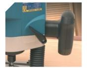
Lever for blocking the routing head, accesible from the handle.
