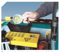
Easy to reload thanks to the special chute. It's equipped with dispenser to reload the glue while working, with no need to stop the machine.
