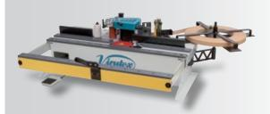
Hot melt glue pot edge bander with automatic rear tape cutting. Foot pedal for curved or shaped pieces.
