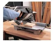
Head can be tilted from 0° to 45°. The machine head can be turned from 0° to 45°.
