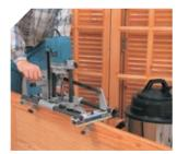
The machine is also able to work horizontally. Especially useful if deciding to make a series of mortises, with the doors unhung.
