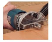
Trimming heads 5600060 and 5646365 are equipped with dust collection nozzle.
