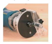
The V3 head includes its own vacuum collector with a brake, and is also supplied with three sliding bases. (Holes d= 20, 26 and 30 mm)
