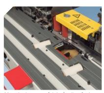
Motorised pressure (gluing) roller. Optimum capacity of the glue pot. Easy to reload and to maintain clean thanks to its Teflon® cover.
