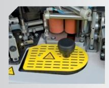
Glue pot with non-stick Teflón® cover. The amount of glue can be also adjusted.
