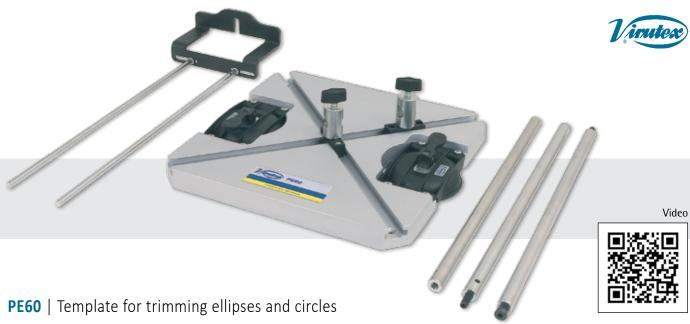
Multiradius template for trimming circular or elliptical forms. Ideal for manufacturing mirrors, windows, doors or any other decorative items by means of an elliptical or circular trimming. The use of the two guide supports (standard equipment) allows the elliptical trimming and the use of only one support allows the circular external trimming or moulding.
