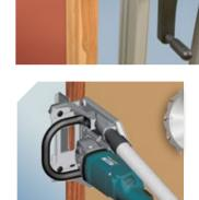
Trimming wooden window frames. Register on the adjustable front guide square.
