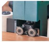
Power trimming unit: trimming both sides simultaneously.
