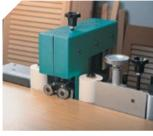
Power trimming unit: Trimming strip on both sides simultaneously.
