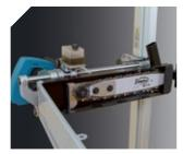
Equipped with an effective chain saw for a clean and easy cut. Fitted with safety protections to avoid any contact with the chain saw, even during the cut.
