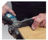
Vacuum connection equipped with a bearing brake to prevent leaving marks on the edge.
