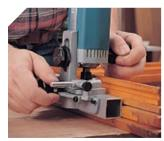
Slotting a window, flashing side.
