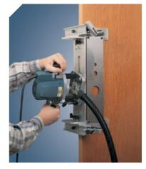
cure, reliable grip. Works horizontally also. UC16K includes a height bar, making possible identical recesses on several doors at the same height, with no need to readjust the lock mortising template holder.
