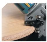
Radius copier (optional). Edge rounding or cutting on radius (R=5, 10 or 15) is also possible using radius blades 9841005.
