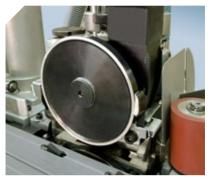
Trimming unit with digital adjustment. Possibility to trim with different radius or  $10^{\circ}$  chamfer. Excellent finishings without adhesive residue due to the double flat scraper. Automatic front and rear flush cutting.
