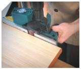
It allows to plane shelves or doors without splintering or damaging the edges.
