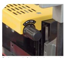
Precise control of the glue dosage on the tape, which helps to adapt correctly the performance of the machine to different kind of materials.
