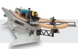
MI250 Tilting table. For gluing panels with a lean from 15° to 50°.
