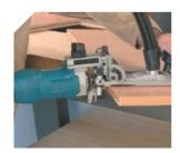
Trimming the edge with the straight bit.
