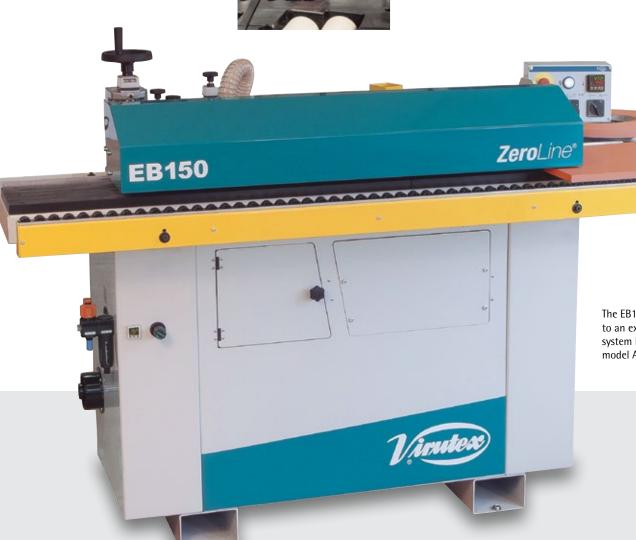
The EB150 must be connected to an external dust collection system like our dust collector model AS382L (optional)
