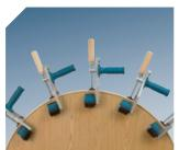
Fixing tapes on convex panels
