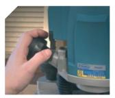
On-Off switch and head blocking may be activated from the knob, giving total, safe control of the machine.
