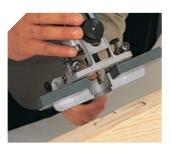
Placing hinges with the ZB93 head.
