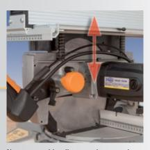
New upper table adjustment by cranted system. Gives a precise and smooth adjustment.
