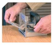
Angle and height of the front fence can be adjusted on a graded scale.
